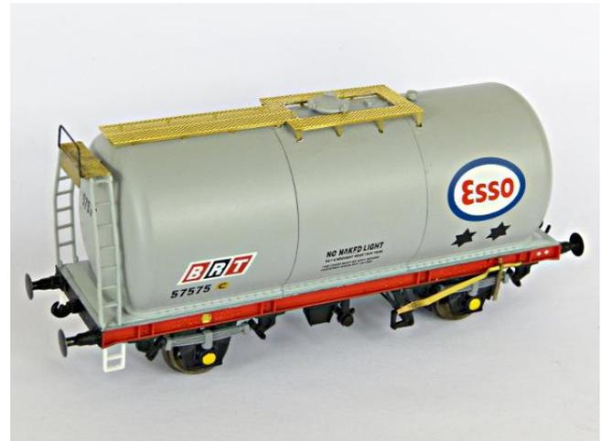
12. Remove the walkway and the end platform. On the end platform there are two holes on either side of the number board for an end handrail and two holes at the rear face. Enlarge and drill out these holes with a 0.5mm Ø drill.
