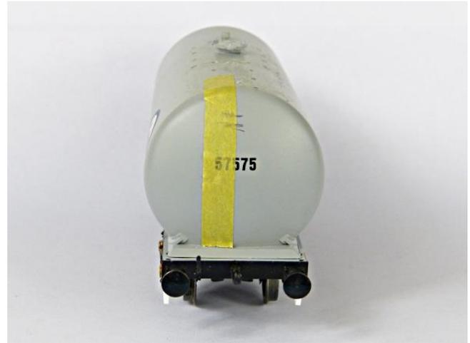
11. Use a pointed implement to mark the position of the holes and drill out with a 1mm Ø drill. Offer the platform assembly to the barrel to ensure the fit is correct.
